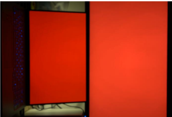
Fig. 3 Condition 3 (High Saturation Red), LEW00005.ARW. ISO 400, monitor displaying #FF0000, 1/45s, f/5.6. Shutter was 1/45s as recorded by EXIF; at this speed minor 60Hz banding may theoretically occur, but was not observed in channel statistics. R
